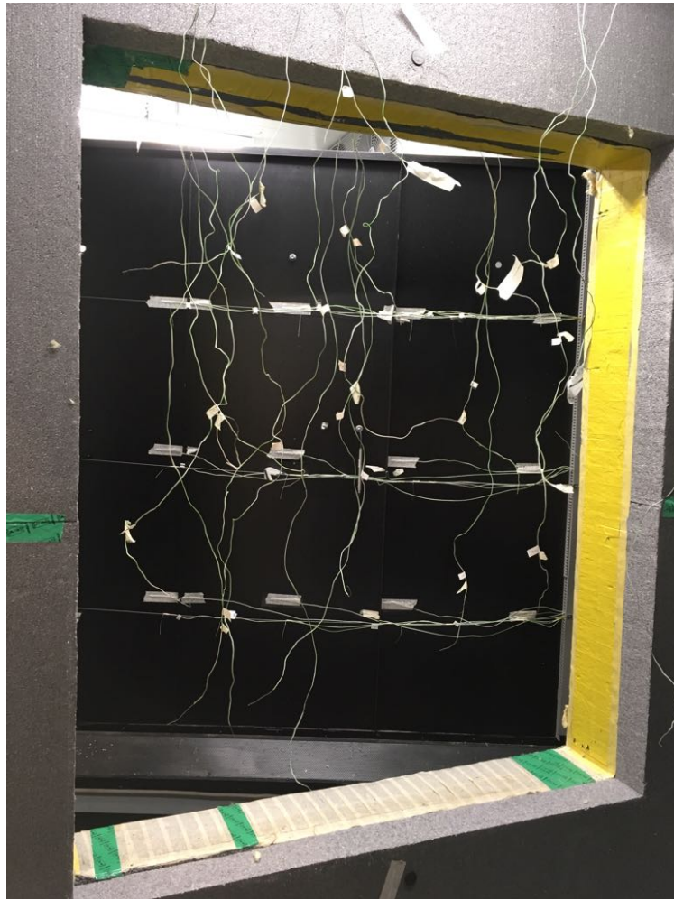
Figure 3.10. extra 100 mm of EPS is attached to the surround wall from the warm side.
