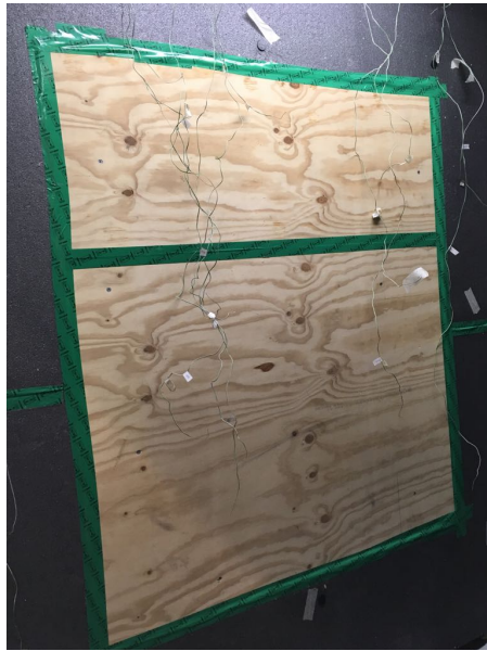
Figure 4.11. Wall specimen is sealed at the edges with high tensile strength tape to increase the air tightness and reduce edge losses.
