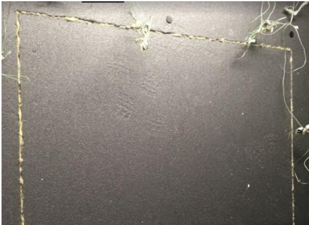
Figure 4.5. Mineral wool is stuffed at the boundary between the surround wall and the specimen to reduce the edge heat loss.
