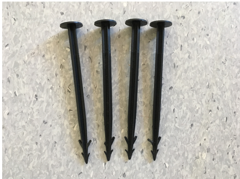
Figure 3.11. Plastic nails used to attach the extra 100 mm EPS layer.
