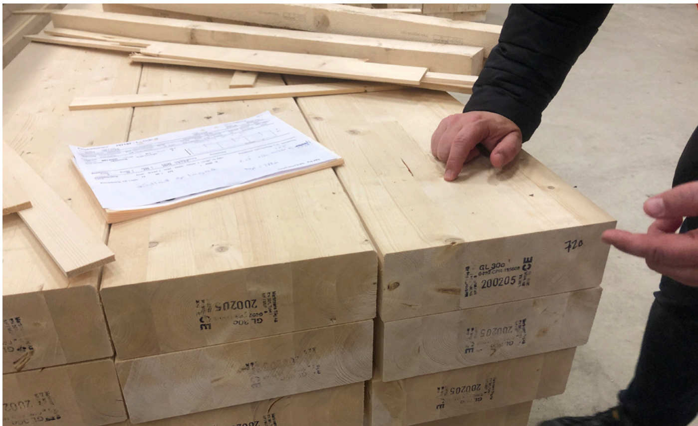
Picture 8. Glulam beams from Martinsson factory in Bygdsiljum, source: authors
