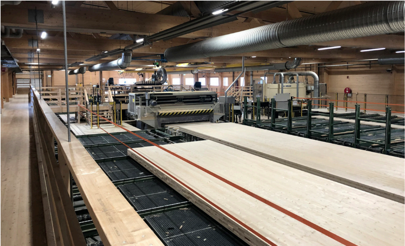
Picture 6. From Martinson's production line of cross laminated timber, Bygdsiljum, source: authors
